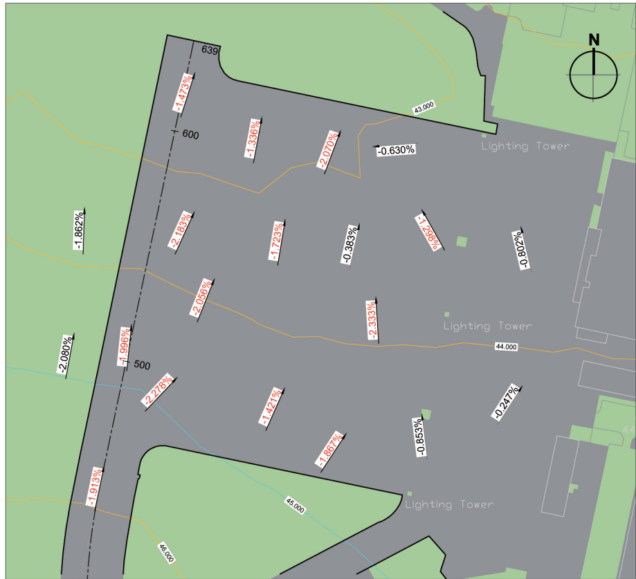
Passenger Terminal Apron - Non-compliance (clause E-360) On an aircraft stand, the maximum slope should not exceed 1% in any direction
